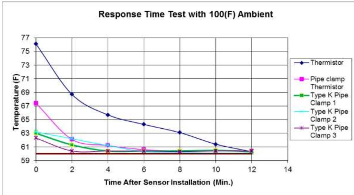
**Figure 1** The response time of the tested refrigerant line temperature sensors in still air was as long as 12 minutes.
