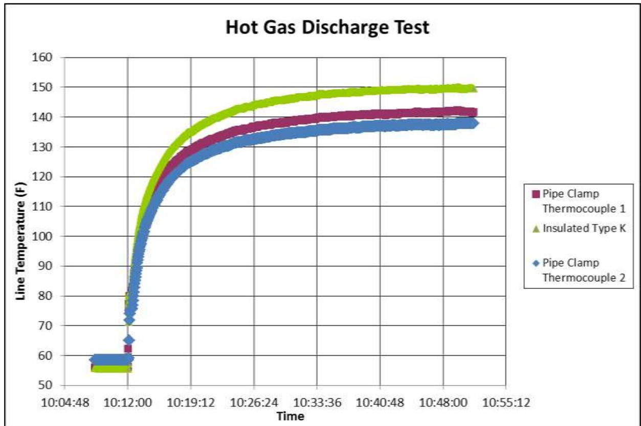
**Figure 2** Pipe clamp thermocouples #1 and #2 produced errors of 8 and 12°F when tested in moving air.
