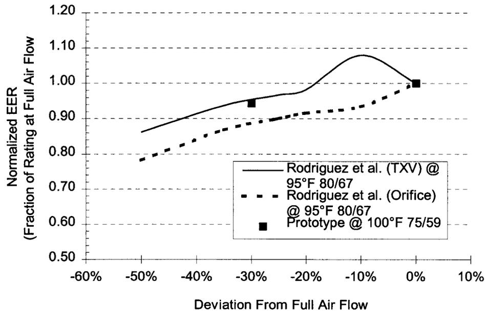
**Figure 3. Indoor Coil Air Flow Effect on EER of Prototype and Other Units**
