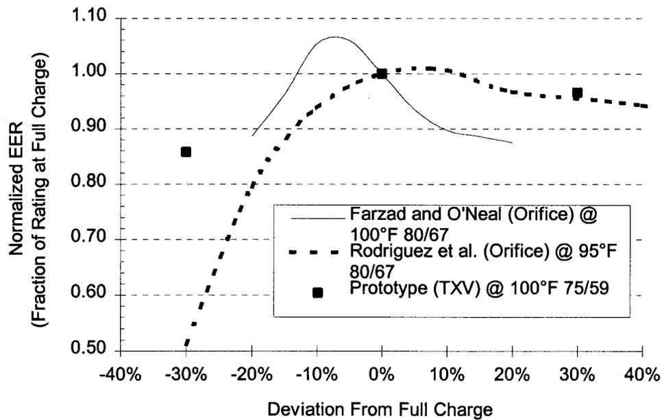
**Figure 2. Charge Effect on EER of Prototype and Fixed Orifice Units**
