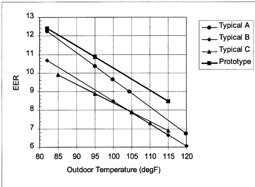
**Figure 4. EER Comparisons for Typical Units and Prototype (80/67°F)**
