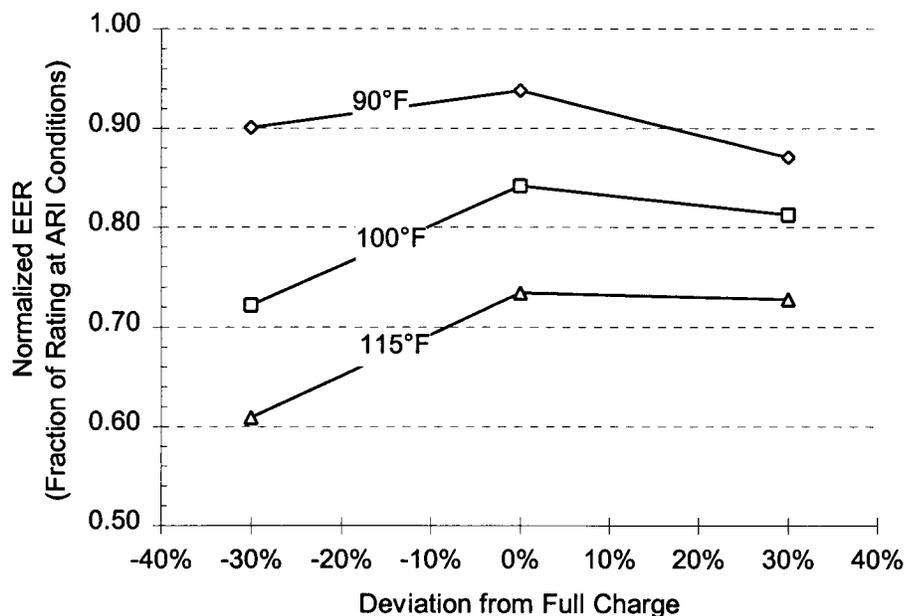
**Figure 1. Charge Effect on Prototype EER.**
